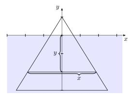
The differential of the hydrostatic force is given by  $dF = \rho g d \, dA$ . From the diagram, we see that d = -y and  $dA = x \, dy$ . By considering similar triangles, we see that
